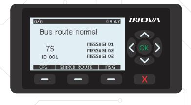
**Round trip mode:** It can contain up to 10 message screens on each column, with numbers from 1 to 999, the messages are separated and can be accessed through the directional keys on the HMI.
