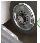
The automatic and permanent balancer is built with a circular tube filled with metallic spheres and a compound of special oils that spread throughout its perimeter balancing automatically and permanently all the moving tires of the vehicle and adapts itself to wear and tear natural tire.
